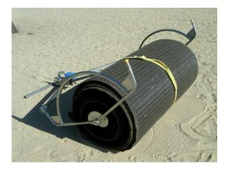
Move the Mobi-roll 'N Stow above the belt until the belt can be placed around the mat. Fasten it with the buckle.
