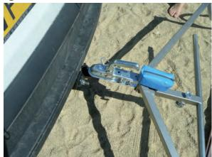
4. Check the Mobi-roll 'N Stow is correctly locked to the vehicle towing bar by lifting it. If it is locked, it will stay on the coupling ball.
