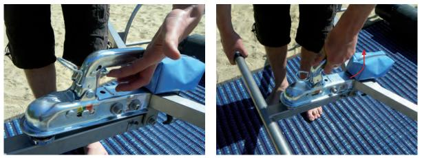
2. Move the manual handle backwards and lock it with the toggle levers
