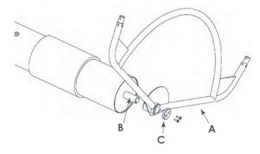
3. Screw the top C with supplied M6 screws, using the Allen key  $n^\circ\,4$
