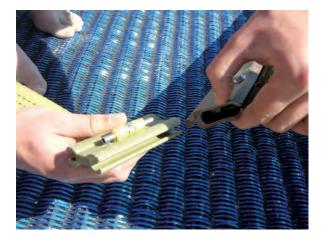
Connect the "X" (strap) with the "C" (mat) and push the X to face the screws.
